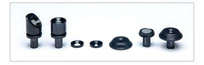
In addition to standard targets, Aligned Vision also offers field-repairable, low-profile targets, which resolve problems created by normal-profile targets. Specifically, low-profile targets may be left in place and not interfere with bagging and other operations. Normal-profile targets often must be removed for such operations. Field repairability represents an economic advantage, since repair costs a small fraction of target replacement costs.
