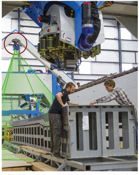
LASERVISION inspects wing spar during production yet independent of production equipment.
