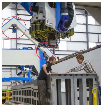
Figure 1. Large-field automatic inspection system mounted to a second gantry over a large AFP cell. Two inspection units are circled in red.
