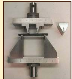
Three and Four Point Flexure ASTM D 790, D 6272, D 7264
